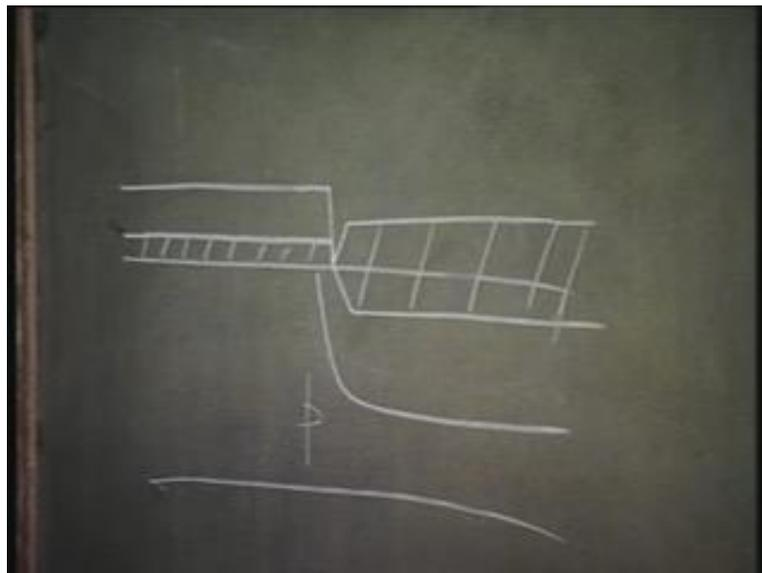
So, I do an oxidation and in the process this arsenic has gone in a little bit, fine. Now, I am going to strip off both the oxide and the nitride.
