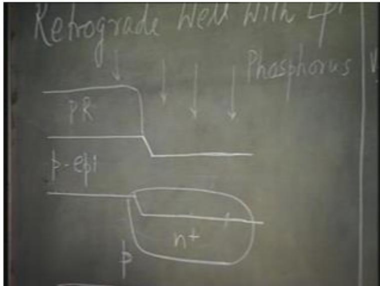
Next step, you just protect this with photoresist and carry out, this time you do a phosphorus implantation, because you want to have a deep n well.
