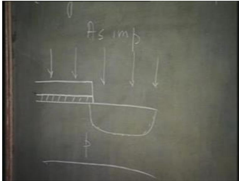
So, to this end, I first protect certain region with an oxide-nitride cap, ok and I do a blanket implant. Ok? One uses arsenic for this blanket implantation, ok because you remember that for all buried layers, you prefer arsenic or antimony rather than phosphorus, because phosphorus will go deep. It actually should not be so deep, so I should have a thinner region, never mind. Ok? Now, after this implantation is over, your next step is to carry out an oxidation, right?
